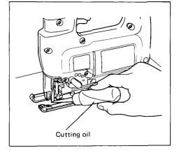
The underside of the workpiece can be greased instead of using a coolant.
